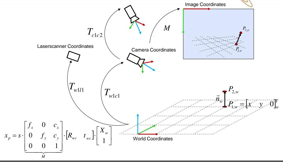
Extrinsic calibration of all cameras and laserscanners using different target devices.
